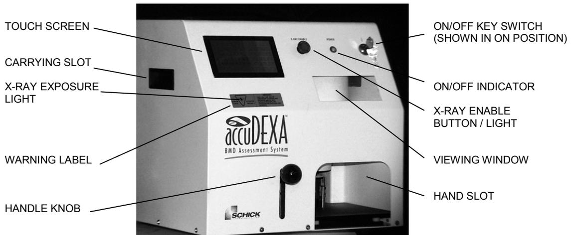
Figure 1. The accuDEXA Device, front view
